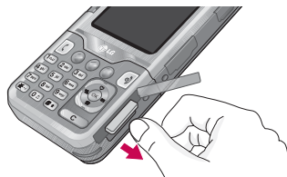
Remove the memory card
